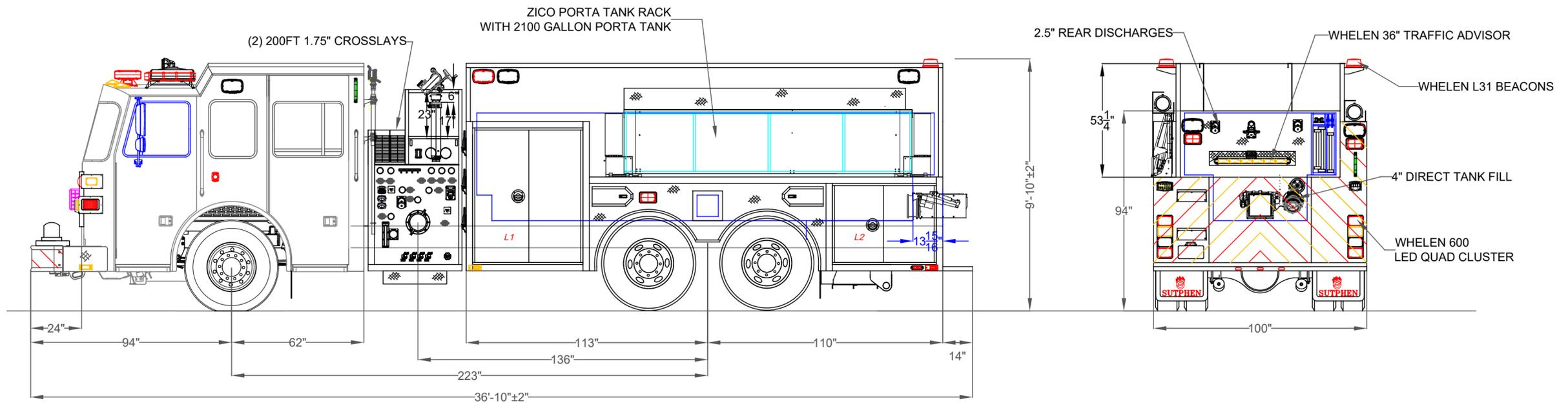
DIMENSIONS SHOWN ON THIS DRAWING ARE APPROXIMATE AND ARE SUBJECT TO MINOR DEVIATIONS DURING CONSTRUCTION.
