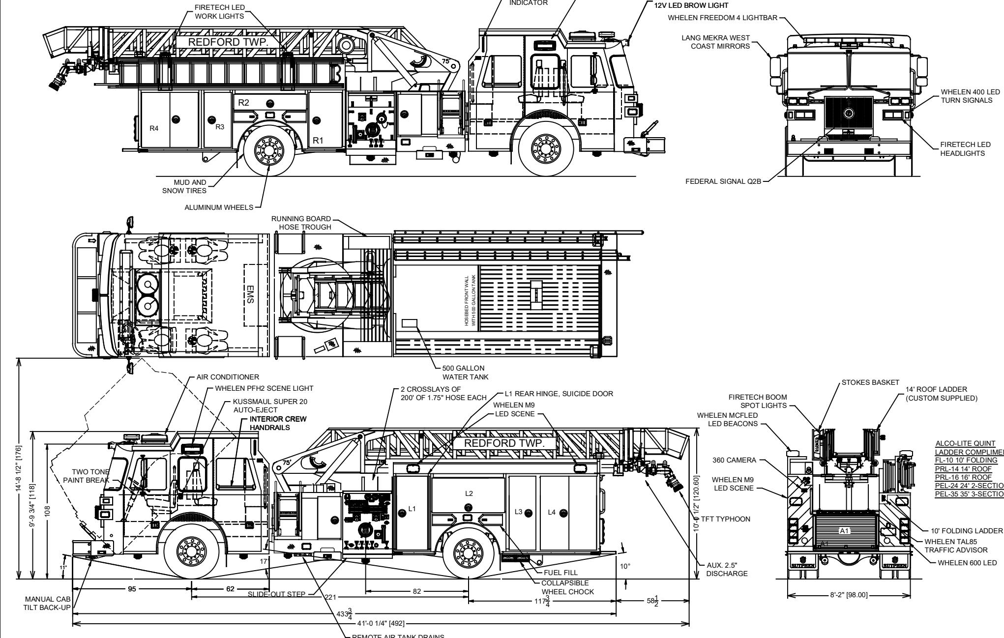
DIMENSIONS SHOWN ON THIS DRAWING ARE APPROXIMATE AND ARE SUBJECT TO MINOR DEVIATIONS DURING CONSTRUCTION.
