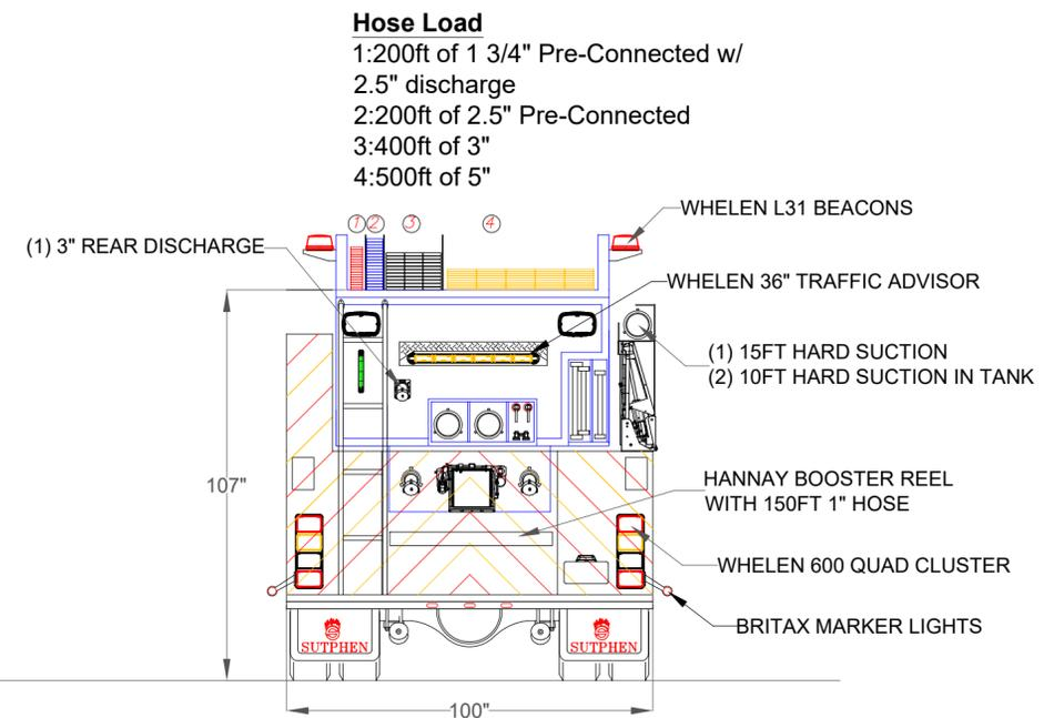
DIMENSIONS SHOWN ON THIS DRAWING ARE APPROXIMATE AND ARE SUBJECT TO MINOR DEVIATIONS DURING CONSTRUCTION.
