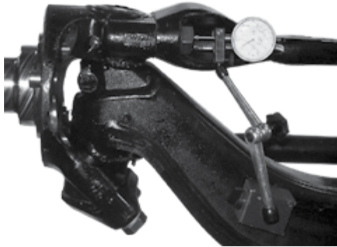
FIGURE 7-11 CHECKING UPPER KINGPIN BUSHING
