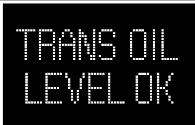
Figure 5–2. Correct Fluid Level Display
