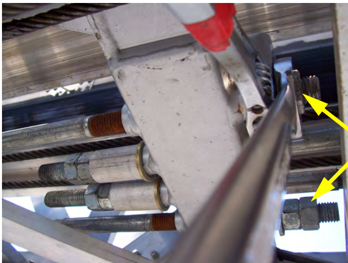
Cables Adjustment - Outer Jam Nut Retighten
