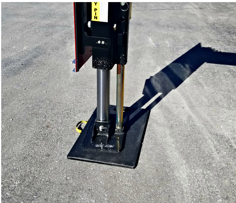
Auxiliary Pad Under Outrigger
