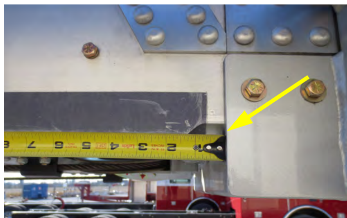
Measuring Point for Other Ladder Sections
