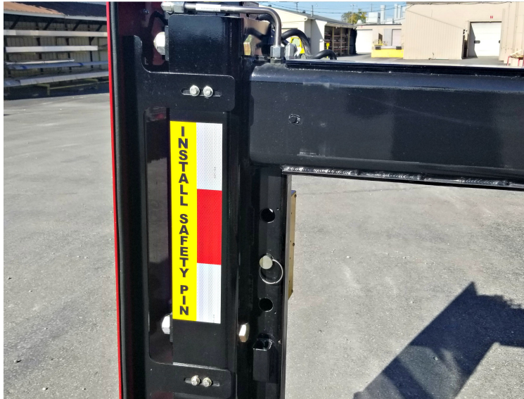
Installed Safety Pin
