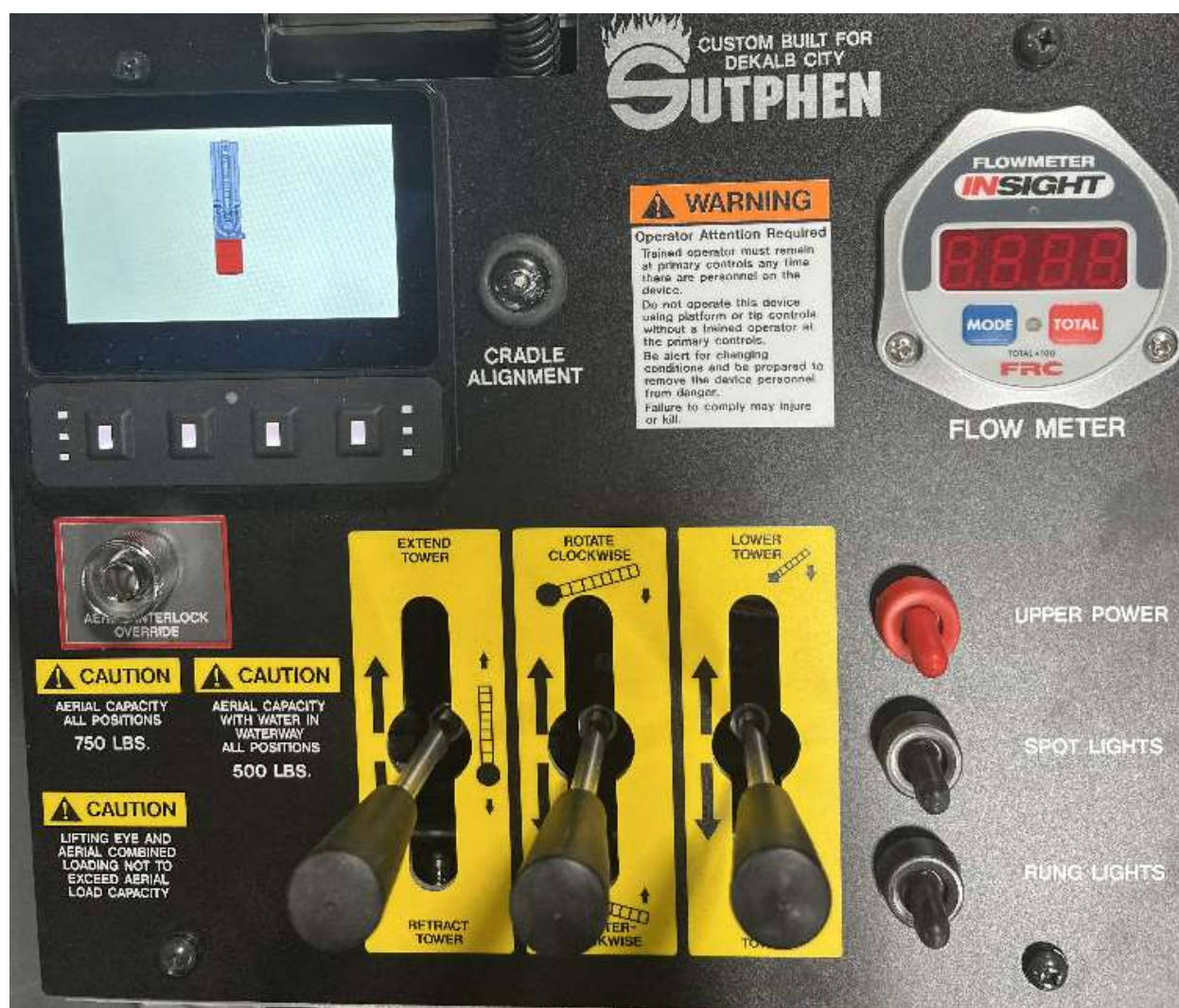
Figure 3- Ladder Controls At Pedestal
