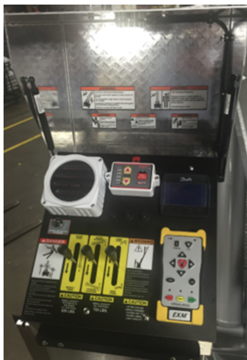
Figure 3 Ladder Controls At Pedestal
