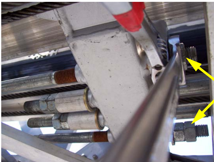
Cables Adjustment - Outer Jam Nut Retighten
