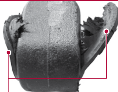
Disconnected Rubber Flange
