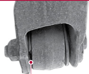
Missing Rubber Flange
