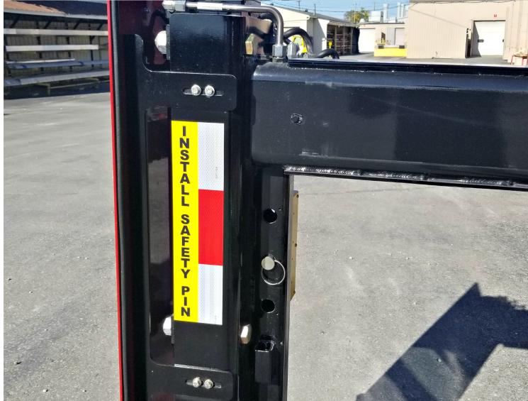
Installed Safety Pin
