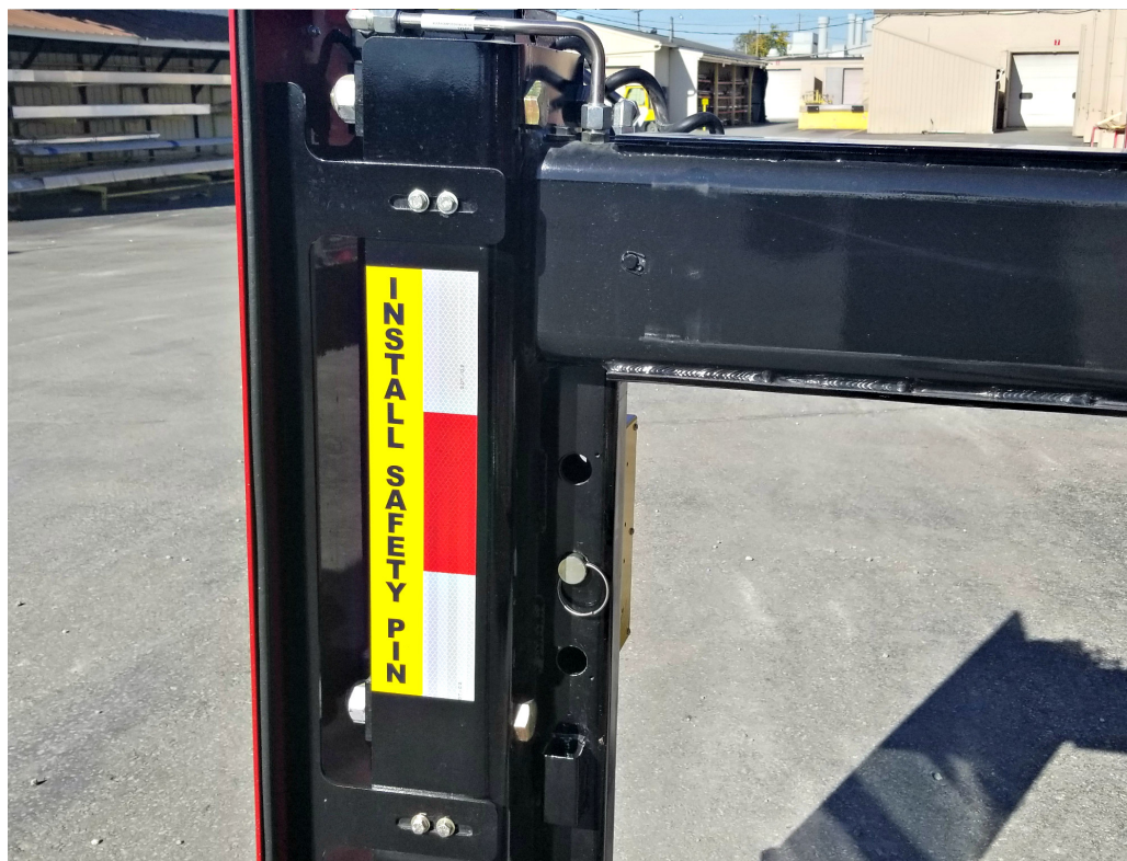
Installed Safety Pin
