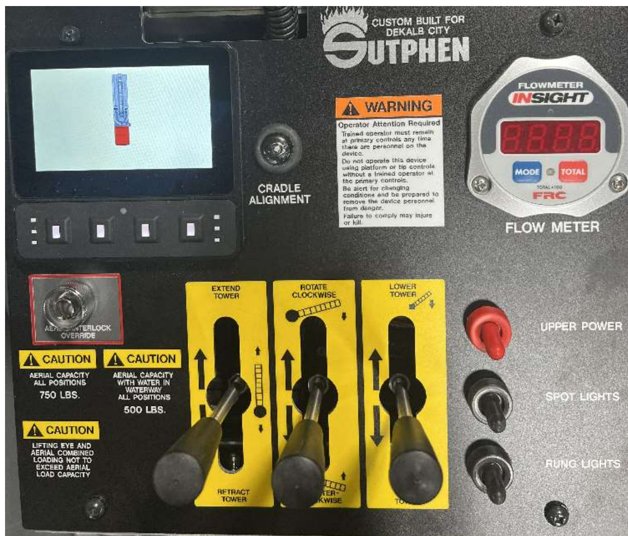
Figure 3- Ladder Controls At Pedestal
