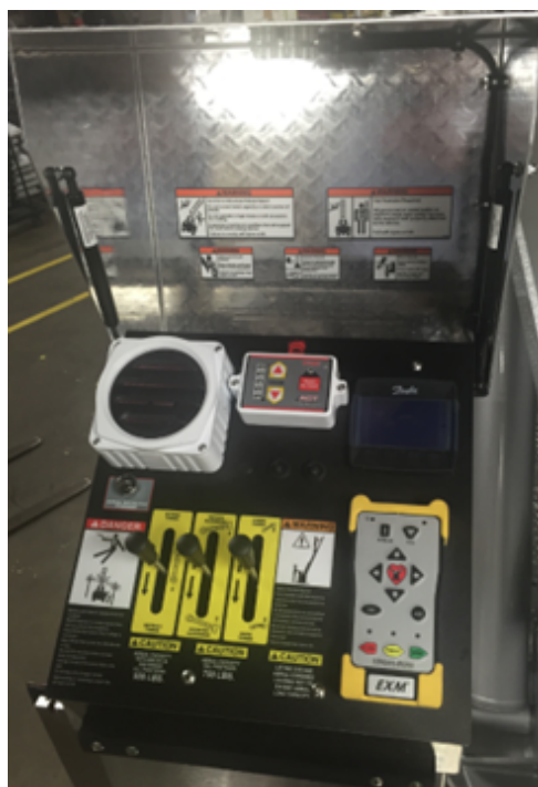
Figure 3 Ladder Controls At Pedestal
