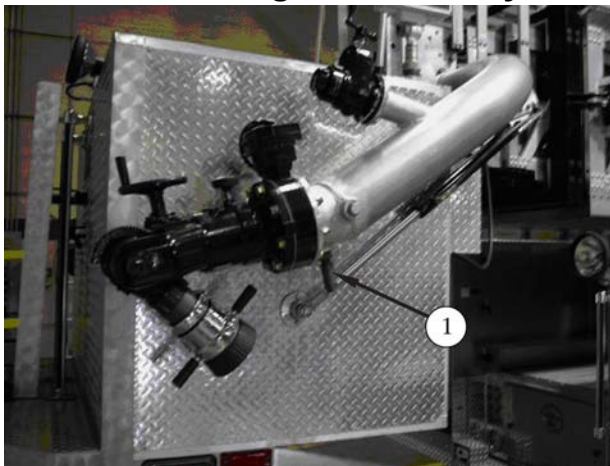
Truck has Automatic Drain Valve on Yoke
