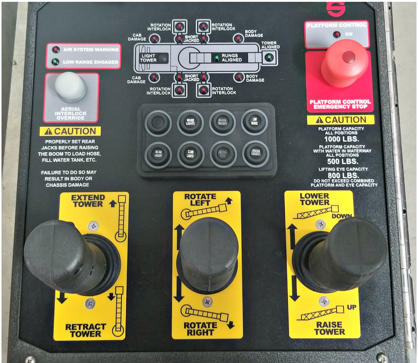
Pedestal Control Panel
